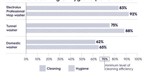
\*\* Amount of bacteria removed displayed in percentage (VAH14). This evaluation is dane through the Wet Abrasion Scrub Tester
